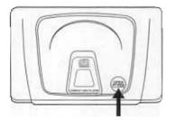
4. Place a CD/CD+G in the compartment tray over the center hub, label side up.
